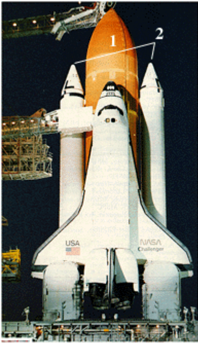
The Challenger on the morning of its final launch. (1) The External Tank. (2) The Solid Rocket Boosters.
