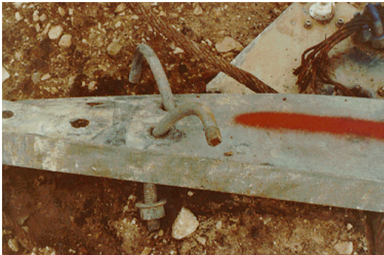
Failed Lifting Bolts:
