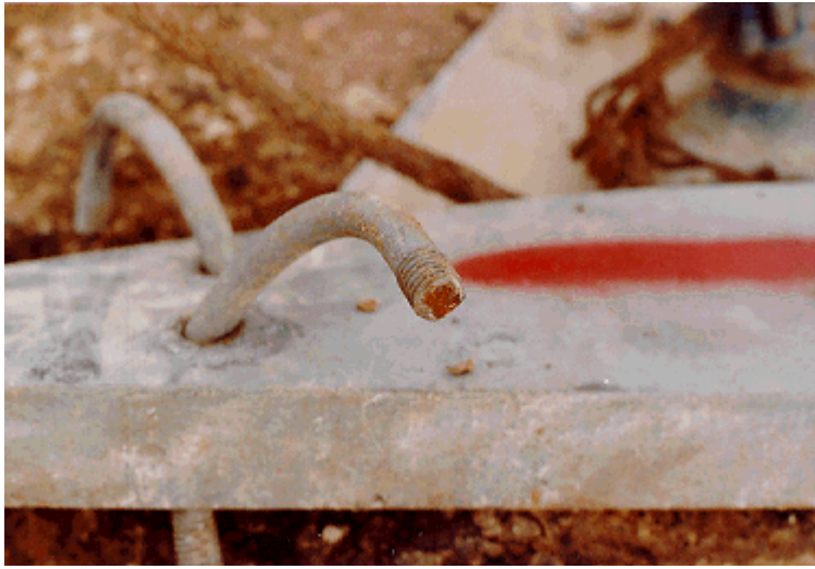
Close-up of Failed U-bolts:
