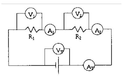
2. Turn the dial on the power supply until the  $V_T$  meter reads 10 V.
